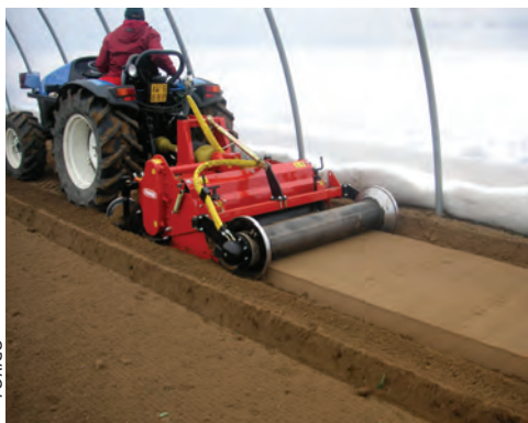
Plate 8 Making raised beds in a greenhouse
