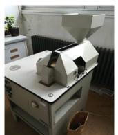
Fig. 5: Laboratory magnetic separator MCC Lilliput
